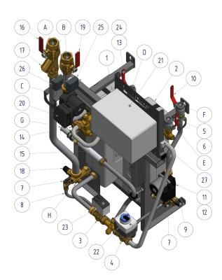
Connections for district heating are welded connections in DN25, for tap water side internal threaded connections in G 1" and for heating side internal threaded connections in G 1 1/2".
